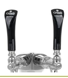
Once the faucet bodies are attached to the tower, thread the handles on to the them. Thread down until the position the handle with curve is facing you, if loose, tighten the black set nut up to the handle base to lock the handle in position. Apply the round sparkling and still water image stickers to the appropriate handles at the top of them.
